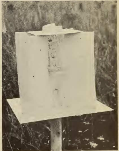
Fig. 2. — Sticky board wing trap used to entrap boll weevils lured by the male sex pheromone. Five virgin male weevils are confined in separate screen cages with food as shown in top center. The synthetic pheromone will replace the male weevils.
